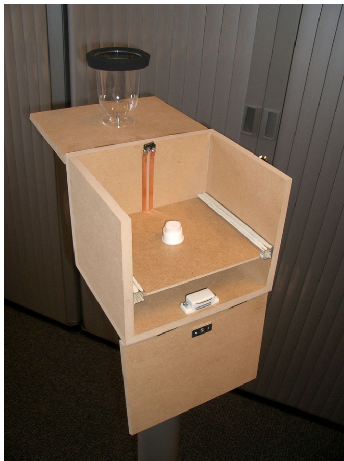
Figure 2 Overview of the interior of a SensaCube in the olfactory condition, showing the Sorbarod attached to the slide and the plastic cup that covered the Sorbarod when the cube was closed.
